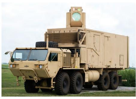
Army S&T is making significant strides to advance HEL weapons, like this one. They have the potential to be a low-cost, effective complement to kinetic energy weapons to address threats from rockets, artillery and mortars, as well as from cruise missiles and UAS.
