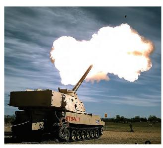
A prototype ERCA Howitzer test bed fires an XM1113 Rocket Assist Projectile. The Army is increasing its lethality overmatch for current and next generation 155 mm systems by developing lightweight armaments with improved accuracy, range and rate of fire.
